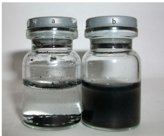
Fig. 2 Images about the dispersion ( 1 \text{ mg mL}^{-1} ) of graphene nanosheets (a) and \text{PMo}_{12} -functionalized graphene nanosheets (b) in aqueous solution
